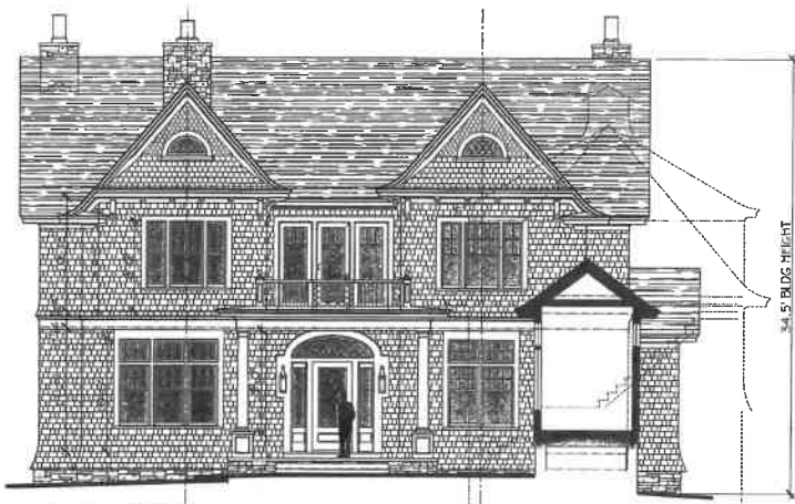
WEST ELEVATION S.C. 1/4" = 1'-0"
