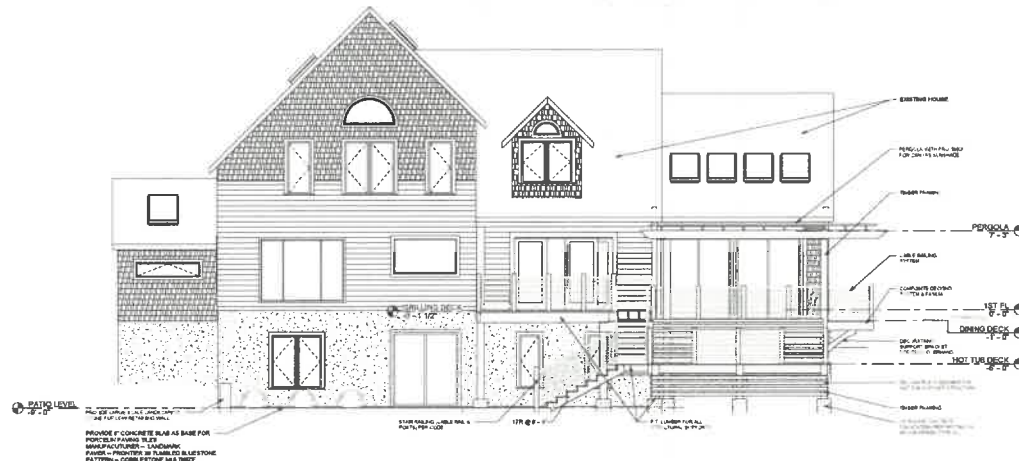
1 SOUTH EXTERIOR ELEVATION 1/4" = 1'-0"
