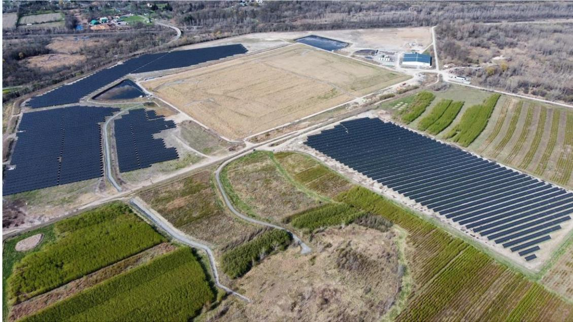
Camillus, NY – 3 x 5 MW Arrays on the Honeywell Settling Basins
