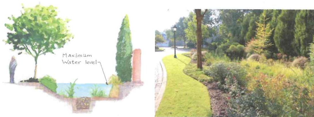
Cross-section of the low-impact stormwater infiltration rain garden designed by Rexford Gonnsen for Villas at Five Points in Athens GA, paired with photo of mature plantings beside the entranceway. The best results occur when these facilities are designed by professionals able to combine landscape architecture and engineering skills.
